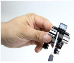
The two screws to remove are located between the battery clips that lock the small right angle bracket
