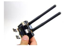
**Step 5**. Insert the battery with the battery power port and the transmitter power port on the same side.
