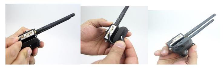
Step 7. Insert the micro HDMI to standard HDMI converter and locking bar assembly into the transmitter micro HDMI input port as shown below.
