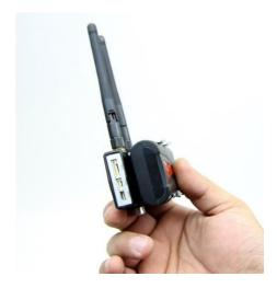
Step 6. Insert the JST connector on the power cable into the power port of the transmitter (note it will click when fully inserted), and insert the barrel plug into the battery.
