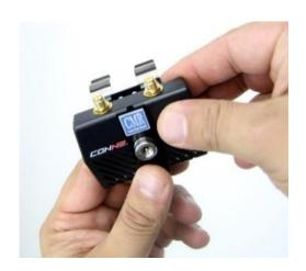
**Step 3.** Position the hole in the small right angle bracket over the small protruding tab on the main mounting bracket. Replace the two screws that were removed in **step 1**., and tighten firmly.
