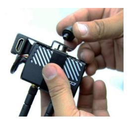
Note: the HDMI locking bar nut also has a ¼-20 tapped hole for mounting the transmitter.
