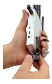
**Step 1.** Screw the battery cage captive thumb screw into the bottom of the 1/4-20 tapped hole on the receiver.
