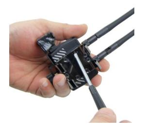
The battery clips can be removed by unscrewing the 4 screws. Save the screws and clips so they can be re-installed later.
