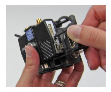
**Step 10.** With the Blackmagic converter mounting bracket on top of the HDMI micro locking bracket, insert the ¼-20 nut and tighten firmly. Note: make sure the Blackmagic converter is pressed up tightly to the support housing while tightening the nut.
