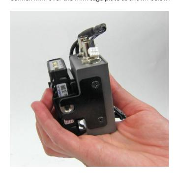
**Step 8.** Plug the D-tap cable JST power cable into the Connex Mini Power port. Press in until it clicks locked.
