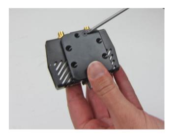
**Step 6**. Insert the voltage converter into the Blackmagic converter bracket as shown below. Note the micro USB cable end should be at the side of the Blackmagic converter micro USB power port. Center the converter in the support bracket
