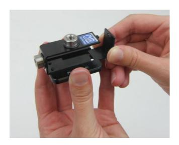
**Step 3.** With the short right angle bracket removed, Slide the support housing over the Connex mini TX. Note the main bracket goes on the Connex Mini side with the Connex logo.
