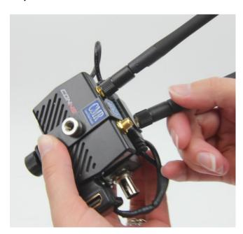
**Step 12.** Insert one end of the HDMI cable into the right angle adapter.
