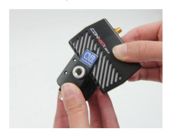
**Step 4.** Position the short right angle bracket over the top of the Connex Mini TX. Press it into place so that the tab on the main bracket snaps into the hole in the short bracket.
