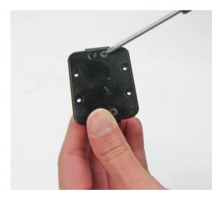
$\label{eq:Step 2.} \textbf{Step 2.} \ \ \text{Remove the short right angle bracket}.$
