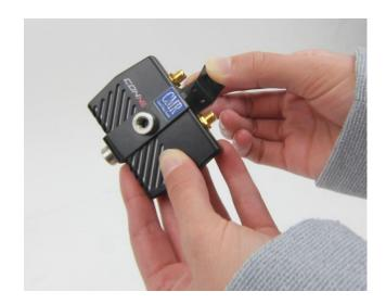
**Step 5** Position the housing in the center of the Connex Mini TX (center the short right angle bracket between the antenna connectors). Insert the two screws removed in step 1, and tighten to secure the housing.
