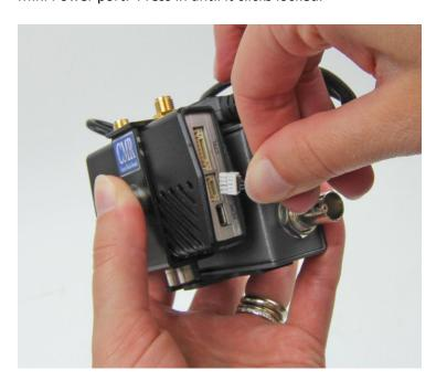
**Step 9.** Insert the HDMI micro locking bracket into the micro HDMI port on the Connex Mini.
