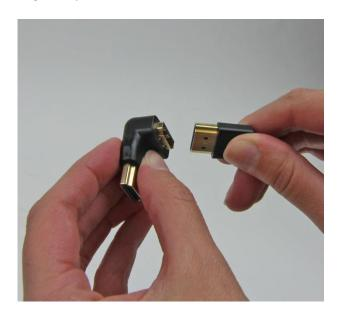
**Step 13**. Plug in the voltage converter micro USB connecter to the Blackmagic power input port. Plug The right angle HDMI connector into the HDMI port.
