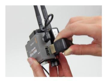
**Step 14.** Plug the other end of the HDMI cable into the full size HDMI port.
