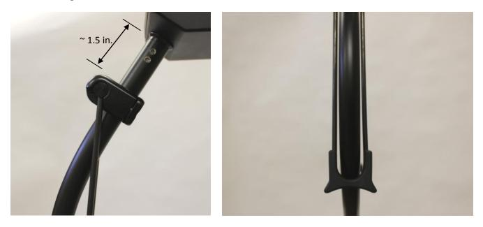
The resting stand should be folded down for normal flying and flipped up to set down the Blackbird.
