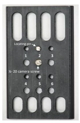
Place the <sup>1</sup>/<sub>4</sub>-20 camera screw in the hole that you think will locate the center of gravity of the camera directly over the gimbal. Or just start with the #2 hole in the middle of the camera mounting plate and check balance. The locating pin screws into the appropriate hole.
