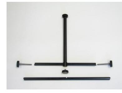
Remove the counterweight screws that are on the present bar you are using and set them aside. Remove the horizontal bar screw and set it aside. Slide out the horizontal bar. Insert the new bar and line up the tapped hole through the bottom of the T-joint. Screw the horizontal bar screw back in to secure the bar. Re-insert the counterweight screws on the new bar.
