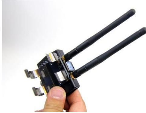
**Step 5.** Insert the battery with the battery power port and the transmitter power port on the same side.
