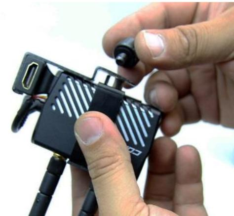
Note: the HDMI locking bar nut also has a ¼-20 tapped hole for mounting the transmitter.
