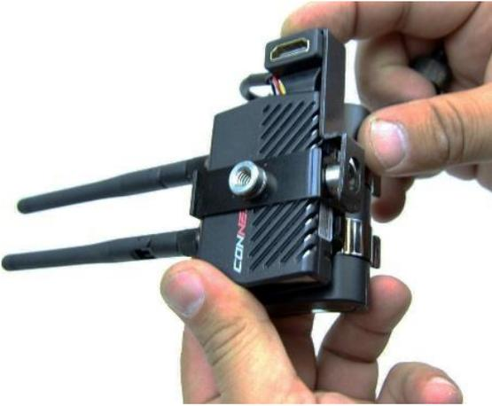
Secure the locking bar with the ¼-20 nut, **and tighten securely.**
