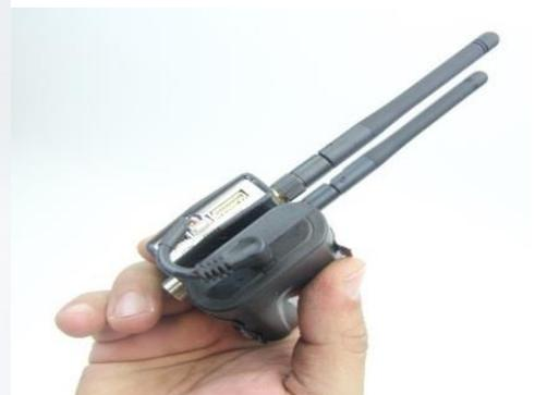
**Step 7.** Insert the micro HDMI to standard HDMI converter and locking bar assembly into the transmitter micro HDMI input port as shown below.
