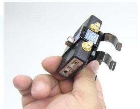
**Step 4.** Attach the provided rod antennas to the Connex Mini transmitter by screwing them on.
