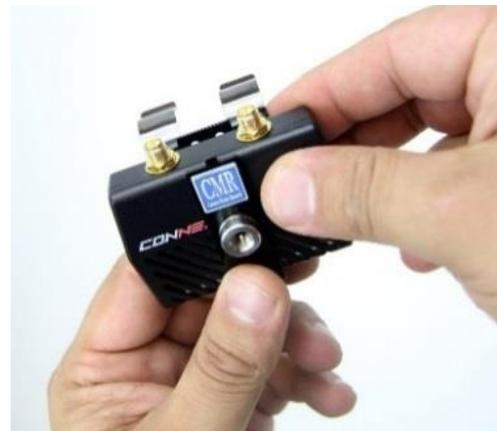
**Step 3.** Position the hole in the small right angle bracket over the small protruding tab on the main mounting bracket. Replace the two screws that were removed in **step 1.**, and tighten firmly.
