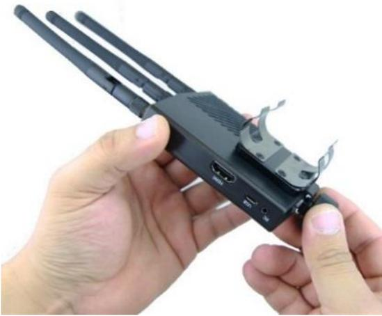
**Step 1.** Screw the battery cage captive thumb screw into the bottom of the ¼-20 tapped hole on the receiver.
