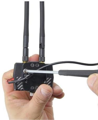
The D-tap power cable, PN: DT15 must be purchased separately. It includes a strain relief which can be mounted to the Mini transmitter cage as shown left if the battery clips have been removed.
