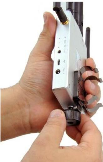
**Step 1.** Screw the battery cage captive thumb screw into the bottom of the ¼-20 tapped hole on the receiver.
