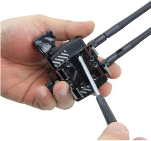
The battery clips can be removed by unscrewing the 4 screws. **Save the screws and clips so they can be re-installed later.**
