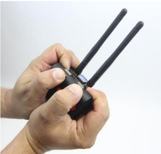
This applies to both the transmitter and the receiver. Hold the cage in your hands so that you have a grasp of the cage and the battery. Use your thumbs to press up on the clips and your index fingers to push out on the battery. Remove battery.
