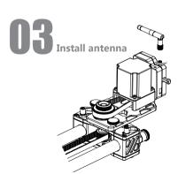
After installing the motor section, turn the antenna on the antenna base clockwise.
